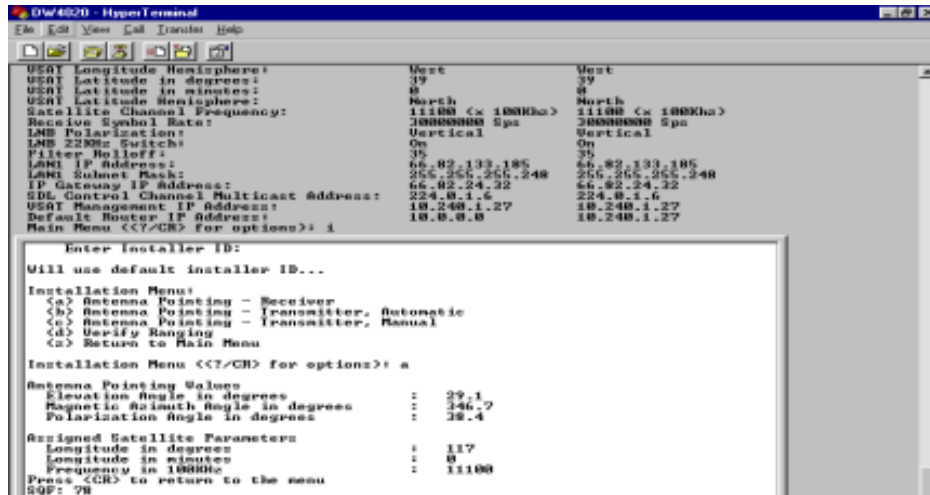
Figure 82: Antenna Pointing - Receiver
